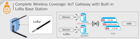
Connect large volumes of low-cost sensors using unlicensed LP-WAN backhaul to dramatically reduce CapEx and OpEx.
