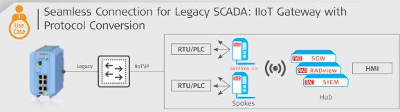
Enable brownfield deployments with built-in conversion or third-party, container-based software. Connect legacy SCADA, NG SCADA and cloud-based IIoT systems, using the following:
